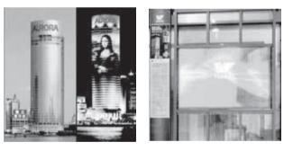
A video curtain wall is a combination of a curtain wall and LED video control technology. With an LED screen applied to its surface, the curtain wall can achieve various visual and audio effects using the curtain wall's display and audio control system.
